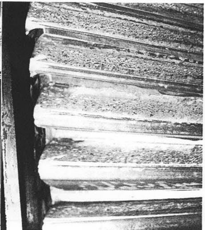
Fig. 3: Gear wheel of 5th transmission step with extensive pitting
